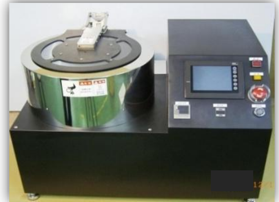
8吋旋轉塗佈/貼合/IR烘乾多功能塗佈機 8in spin-coating/bonding/IR-baking multifunctional coater
