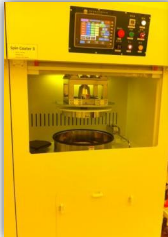
200x200mm有機TFT開發試產用 For 200x200mm OTFT R&D
