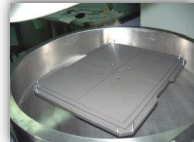
320x400mm玻璃基板光阻塗佈用 For 320x400mm glass PR coating
