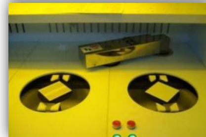
100x100mm陶瓷基板光阻塗佈用 For 100x100mm ceramic PR coating
